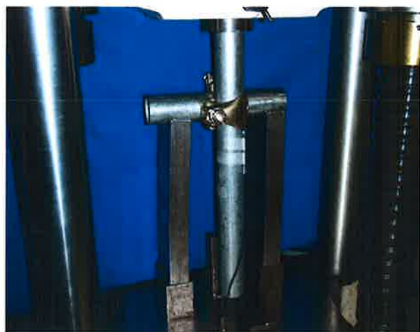
Photograph of setup for Indentation Check
