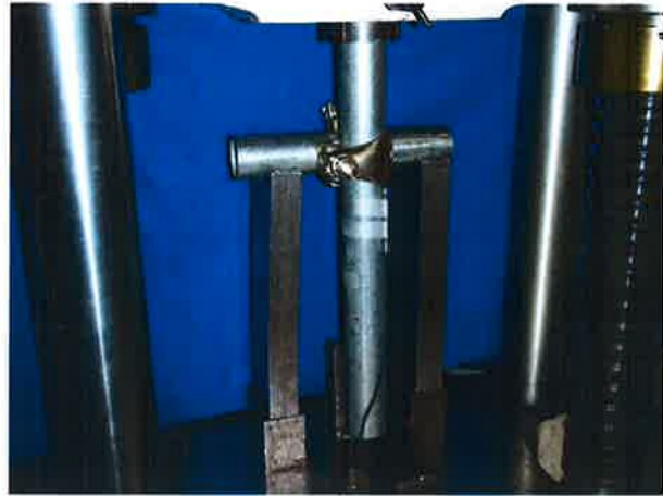
Photograph of Setup for Slipping Force
