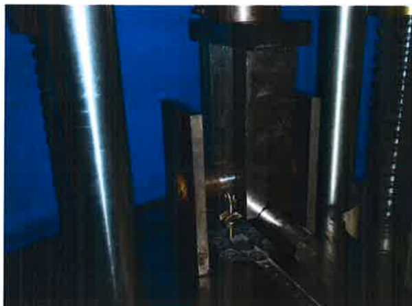
Photograph of setup for Pull Apart Force
