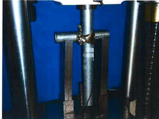
Photograph of Setup for Slipping Force
