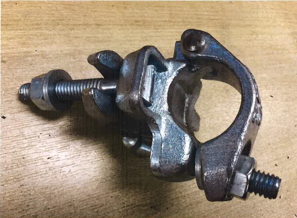
Photograph of coupler under test
