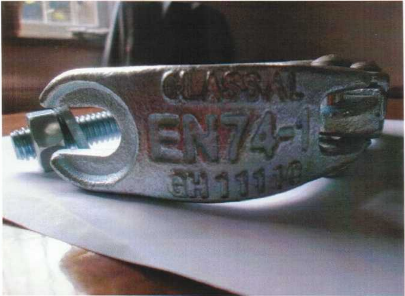
Photograph of markings on the coupler
