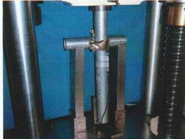
Photograph of Setup for Slipping Force
