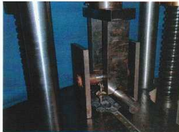
Photograph of setup for Pull Apart Force
