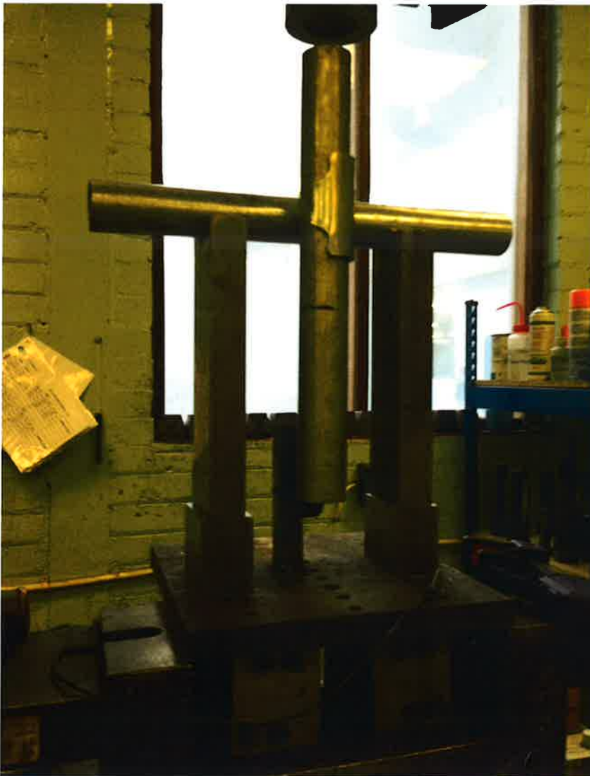
This picture shows the setup for slip test on single couplers but is not necessarily the coupler under test.
